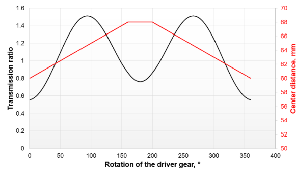
Figure 7. Transmission ratio and center distance variation
