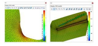
A 2D FEM calculation is sufficient to determine the tooth root stress caused by grinding notches. A 3D
