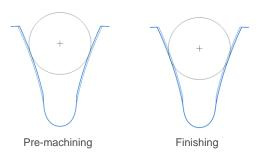
A flattened measuring ball can be defined for spline profiles, to prevent the tooth root from being touched. In the case of deep tooth forms, the ball or roller diameter is automatically calculated to take a correct measurement outside the tip circle.
