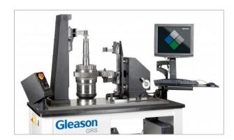
Preferably, the use of existing master gears is targeted. The master gears can be entered in KISSsoft and the rolling with the production gear can be analyzed. The roll testing can be done on a Gleason roll testing machine.
