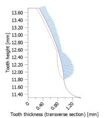
Wear is displayed either in 2D or in 3D and can provide a clear evaluation of the various modifications involved, e.g., the effect of tip relief on wear behavior.
