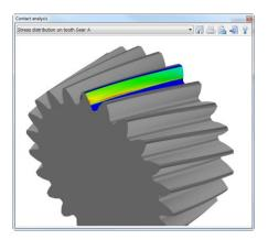
Other graphics show the normal force during meshing, PPTE, the stress in the root area and additionally the distribution of the Hertzian pressure on the tooth flank.
