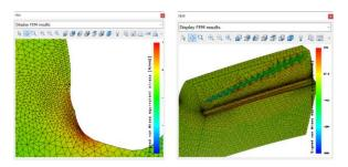
A 2D FEM calculation is sufficient to determine the tooth root stress caused by grinding notches.
