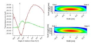
The loaded tooth contact analysis shows the behavior under load, such as stress distribution and contact pattern. The transmission error (PPTE) is used to analyze the noise excitation of gears.
