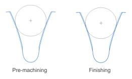
A flattened measuring ball can be defined for spline profiles, to prevent the tooth root from being touched.
