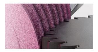
Both grinding processes – profile and threaded wheel grinding – are simulated in KISSsoft and the resulting root rounding is graphically displayed.
