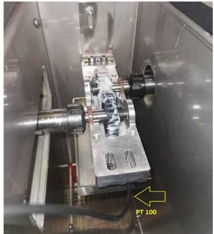
Figure 3: PT 100 sensor inserted for grease temperature control.
