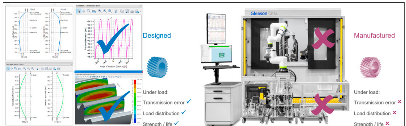
Figure 1—Left, designed gear: Assessment of performance parameters such as transmission error, load distribution or strength is possible considering micro geometry, using LTCA. Right, manufactured gear: Assessment of the same performance parameters is practically impossible in a manufacturing environment.
