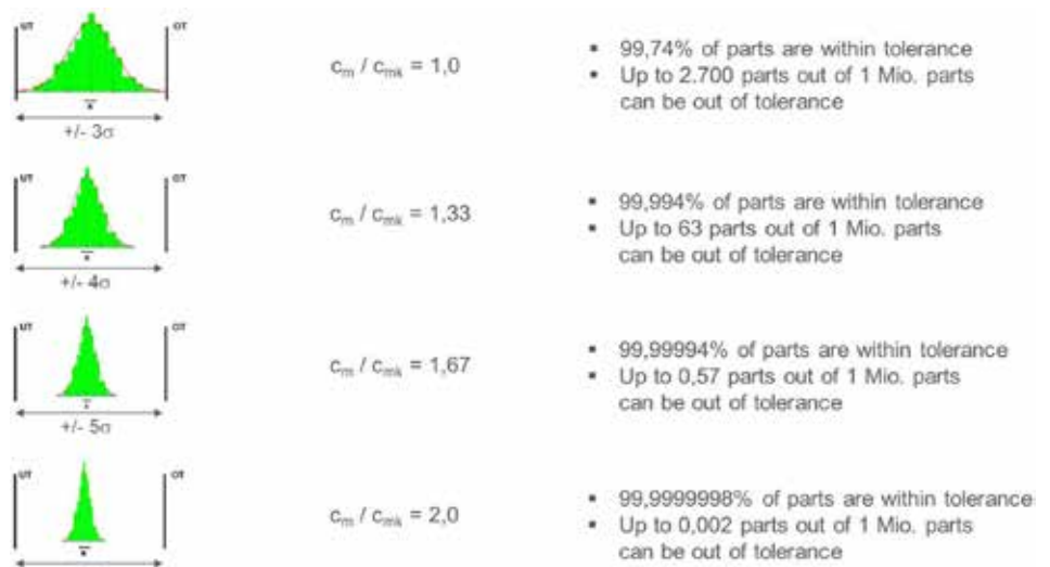
Figure 8: Influence of capability values on probability to match the tolerance.
