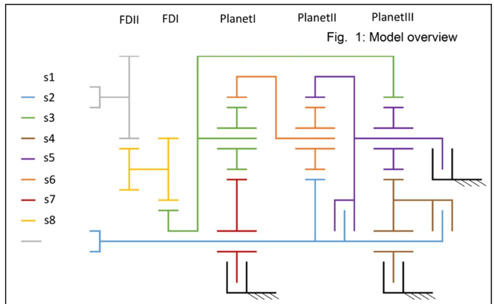
Figure 2 Shafts definition.
