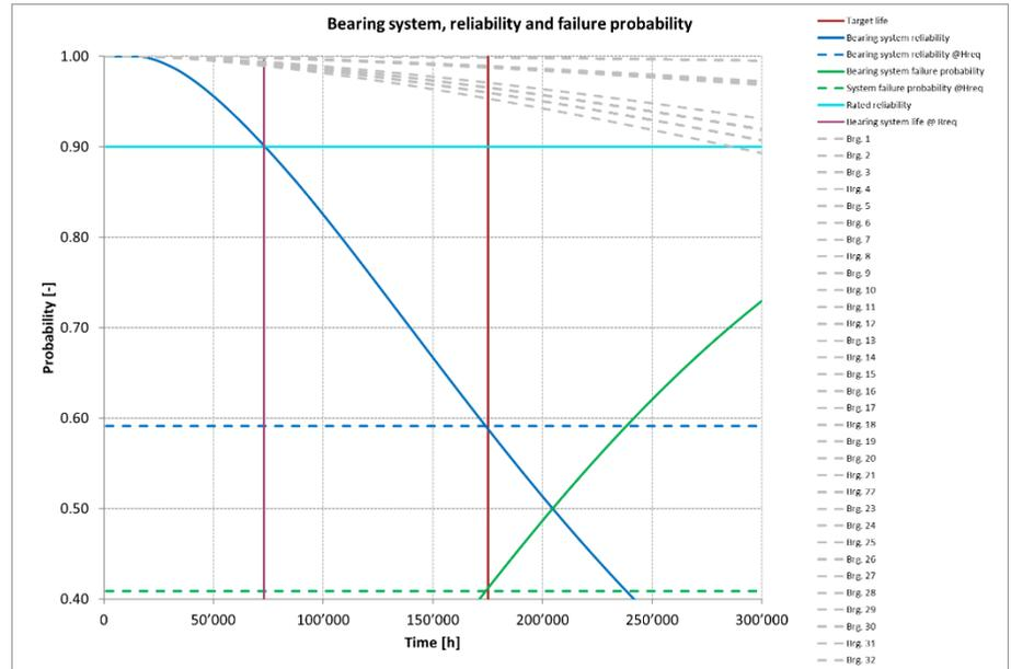
Figure 2 Bearings reliability (grey), subsystems reliability (blue), required subsystems life  $H_{req}$  (vertical, red), rated reliability (horizontal, cyan), subsystem reliability at required life (horizontal, dashed blue), subsystem life at rated reliability (vertical, pink).
