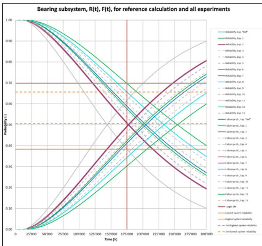
Figure 3 Bearing subsystem reliability for different experiments (blue: reference calculation, green: highest result, pink: second lowest result, grey: lowest result, cyan: second highest results, white: other results). Upper image: reliability curves. Lower image: reliability levels at Hreq.
