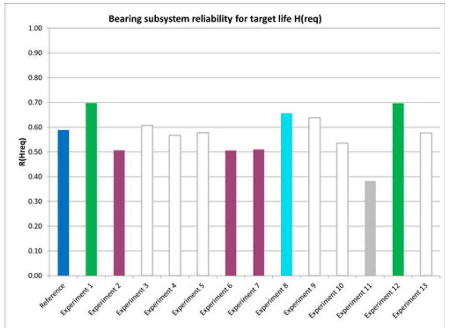
**Figure 3** Bearing subsystem reliability for different experiments (blue: reference calculation, green: highest result, pink: second lowest result, grey: lowest result, cyan: second highest results, white: other results). Upper image: reliability curves. Lower image: reliability levels at Hreq.
