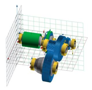
The system deformation is visualized. This helps to understand key contributions to gear misalignment, be it bearing, shaft, gear body or housing deflection.
