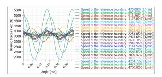
The forced response analysis considers excitation from the transmission error in all gear meshes, shaft imbalance and torque ripple. Time dependent bearing forces allow for calculation of housing noise.
