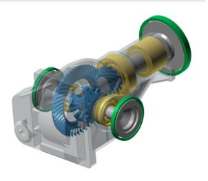
Whatever topology is defined in the sketcher or tree structure of the model and whatever gear and shaft details are designed, the 3D viewer allows for a fast check of the arrangement and use of design space.
